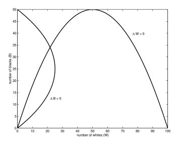
Recognizing that the vertical axis is also a W-nullcline, and that the horizontal axis is also a B-nullcline, this diagram reveals four steady states. Three lie along the edge of the diagram at  $(W^* = 100, B^* = 0)$ ,  $(W^* = 0, B^* = 50)$ , and  $(W^* = 0, B^* = 0)$ . The final steady is determined by the intersection of the quadratic nullclines at  $(W^* = 21.74, B^* = 34.03)$ .
