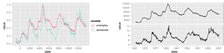
Fig. 9.5: When the series have very different scales we have two alternatives: left, rescale the variables to a common scale, or right, display the variables on separate facets and using free scales.
